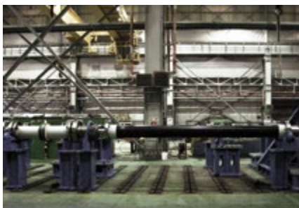
Carbon Fibre Shaft combined with LAMIDISC® coupling.
