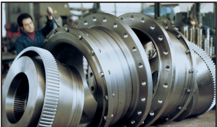
Main Drive Gear Coupling
