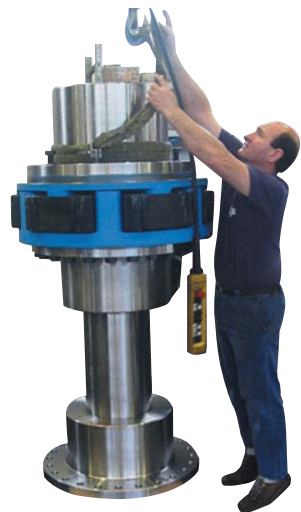
MT Crowned Tooth Gear Coupling. (Nominal Torque up to 7.000 kNm)
