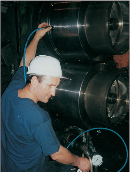
Pumping oil into a spindle with Safeset®
